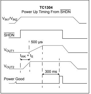
FIGURE 4-3: TC1304 Power-up Timing from SHDN.
