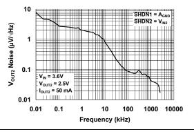
FIGURE 2-35: V<sub>OUT2</sub> Noise vs. Frequency.
