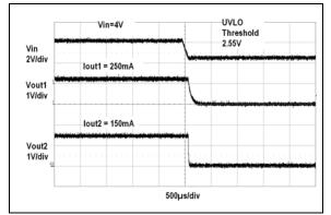
**FIGURE 2-40:** V<sub>OUT1</sub> and V<sub>OUT2</sub> Shutdown Waveforms.
