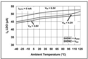
*FIGURE 2-4: I*<sub>Q</sub> LDO Current vs. Ambient Temperature.
