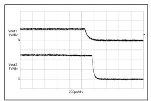
FIGURE 2-43: Shutdown Waveforms (TC1304).
