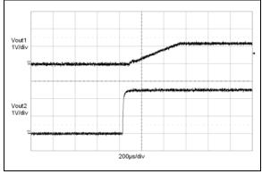
FIGURE 2-42: Start-up Waveforms (TC1304).
