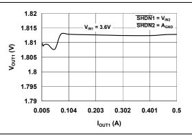
**FIGURE 2-12:** V<sub>OUT1</sub> vs. I<sub>OUT1</sub> (V<sub>OUT1</sub> = 1.8V).
