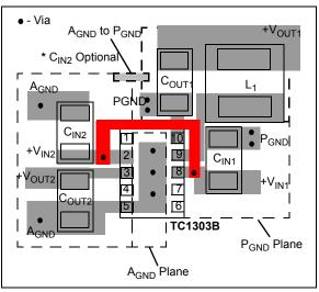
FIGURE 5-2: Component Placement, Fixed 10-Pin DFN.
