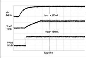
FIGURE 2-39: V<sub>OUT1</sub> and V<sub>OUT2</sub> Start-up Waveforms.
