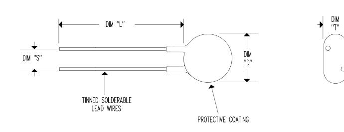
RESISTANCE @ +25°C = 33  $\Omega$  ± 20% MAXIMUM STEADY STATE CURRENT = 1 AMP RESISTANCE @ Imax = 1.075  $\Omega$  NOMINAL
