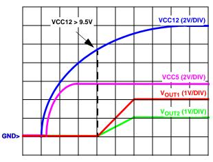
FIGURE 1. 12V POWER-UP INTO SOFT-START
