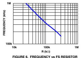
The switching frequency of the ISL6549 is determined by the value of the FS resistor. The graph in Figure 6 shows the
