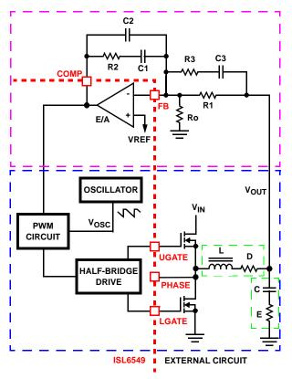
FIGURE 10. VOLTAGE-MODE BUCK CONVERTER COMPENSATION DESIGN
