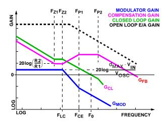
FIGURE 11. ASYMPTOTIC BODE PLOT OF CONVERTER GAIN
