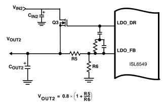
FIGURE 8. OUTPUT VOLTAGE SELECTION OF THE LINEAR  $(V_{\mbox{OUT2}})$
