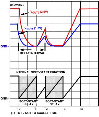
FIGURE 4. UNDERVOLTAGE PROTECTION RESPONSE
