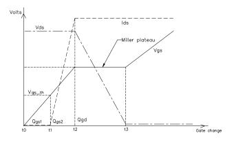
Figure 6. MOSFET switching characteristics Where,
