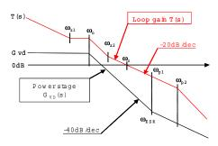
Figure 8. Asymptotic diagram of buck power stage and its compensated loop gain.
