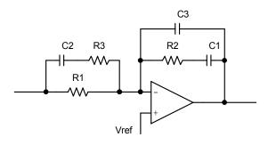
Figure 7. Voltage Mode Buck Converter Compensation Network
