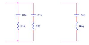
Figure 2. Equivalent RC branch.
