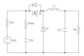
Figure 3. A simple model for the converter input
