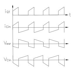
Figure 4. Typical waveforms at converter input. It can be seen that the current in the input capacitor pulses with high di/dt. Capacitors with low ESL should be used. It is also important to place the input capacitor close to the MOSFET's on the PC board to reduce trace
