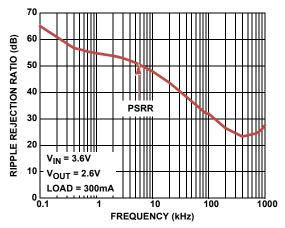
FIGURE 19. RIPPLE REJECTION RATIO vs FREQUENCY
