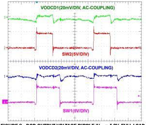
FIGURE 9. DCD OUTPUT VOLTAGE RIPPLE ( $V_{\mbox{\footnotesize IN}}$  = 4.2V, FULL LOAD AT DCD1 AND DCD2)
