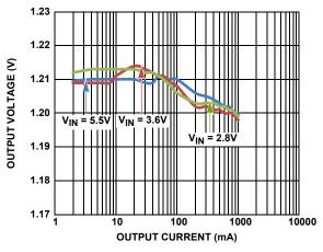
FIGURE 16. DCD OUTPUT VOLTAGE vs LOAD (V<sub>OUT</sub> = 1.2V, PFM/PWM)
