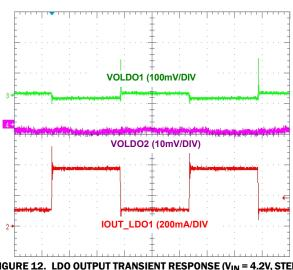
FIGURE 12. LD0 OUTPUT TRANSIENT RESPONSE ( $V_{IN}$  = 4.2V, STEP LOAD: 30mA TO 300mA)
