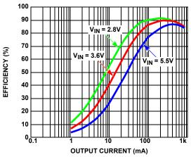
FIGURE 17. EFFICIENCY vs OUTPUT CURRENT (V<sub>OUT</sub> = 1.8V, FORCED PWM MODE)
