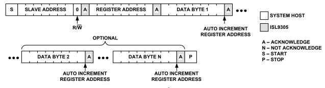
FIGURE 6. I<sup>2</sup>C WRITE
