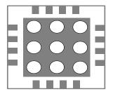
FIGURE 4. EXPOSED THERMAL PAD
