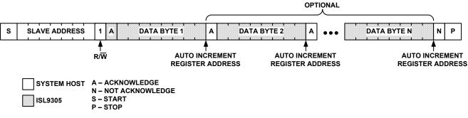
FIGURE 8. I<sup>2</sup>C READ NOT SPECIFYING REGISTER ADDRESS
