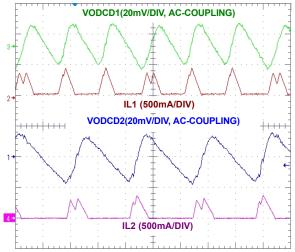
FIGURE 10. DCD OUTPUT VOLTAGE RIPPLE ( $V_{\mbox{\footnotesize{IN}}}$  = 4.2V, PFM MODE)
