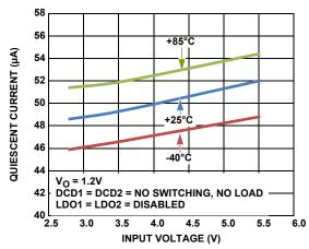
FIGURE 20. QUIESCENT CURRENT vs INPUT VOLTAGE
