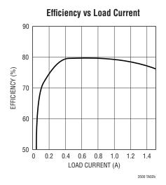
5V/1.5A, 3.3V/0.5A Step-Down with Output Disconnect
