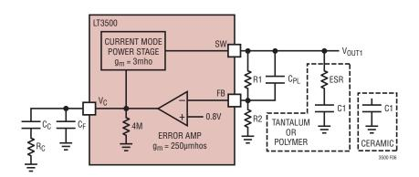
Figure 6. Model for Loop Response
