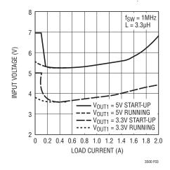
Figure 3. Minimum Input Voltage vs Load Current
