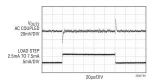
Figure 9. Linear Regulator Transient Response
