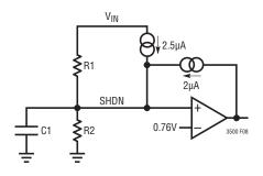
Figure 8. Undervoltage Lockout
