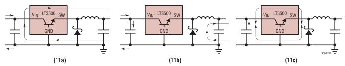
Figure 11. Subtracting the Current when the Switch is On (11a) from the Current when the Switch is Off (11b) Reveals the Path of the High Frequency Switching Current (11c). Keep this Loop Small. The Voltage on the SW and BST Traces will Also be Switched; Keep These Traces as Short as Possible. Finally, Make Sure the Circuit is Shielded with a Local Ground Plane
