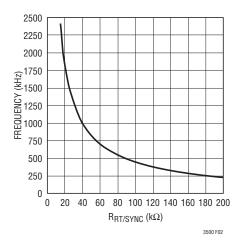
Figure 2. Frequency vs R<sub>T</sub>/SYNC Resistance
