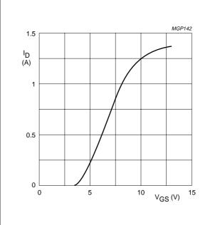
$V_{DS} = 10 \text{ V}; T_j = 25 ^{\circ}\text{C}.$
