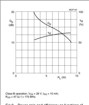
Fig.9 Power gain and efficiency as functions of load power, typical values.
