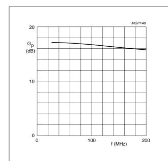
Class-B operation; V<sub>DS</sub> = 28 V; P<sub>L</sub> = 30 W; R<sub>GS</sub> = 47  $\Omega$ ; T<sub>h</sub> = 25 °C.
