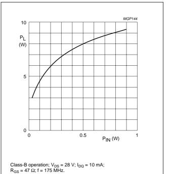
Fig.10 Load power as a function of input power, typical values.
