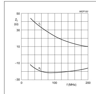
Class-B operation;  $V_{DS}$  = 28 V;  $P_L$  = 30 W;  $R_{GS}$  = 47  $\Omega$ ;  $T_h$  = 25 °C.
