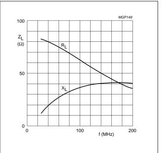
Class-B operation;  $V_{DS}$  = 28 V;  $P_L$  = 30 W;  $R_{GS}$  = 47  $\Omega$ ;  $T_h$  = 25 °C.
