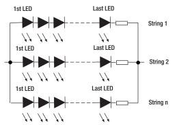
A typical 1W high brightness white LED has a forward voltage of around 3.3V at its operating temperature and draws 350mA. Thus each LED actually draws about 1.15W. Similarly, 3W white LEDs have usually the same forward voltage but can be run at 700mA or more. Using the LED datasheet specification, the optimum LED arrangement and the best driver for each application can be worked out.
