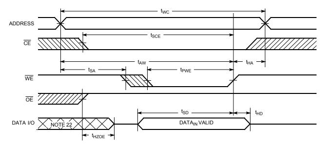
Figure 6. Write Cycle No. 2 (WE Controlled, OE HIGH During Write) <sup>[20, 21]</sup>
