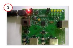
Plug the wall mounted power supply into an AC power receptacle providing power in the range 100 V to 240 V, 50 Hz or 60 Hz. Connect the power supply plug to the hub's 'DC Supply' jack 112.
