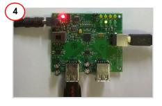
To connect to the PC, plug the USB A to B cable into the hub's 'Up Link' connector P1. Plug the other end of the cable into one of the PC's host controller ports. The hub enumerates as a 'Generic USB Hub'. The hub is now ready for any low speed, full speed, or high speed devices to be plugged into the ports. For the 4-port hub, the board is labeled PORT1, PORT 2, PORT 3, and PORT 4.
