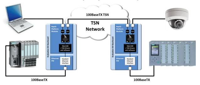
Figure 10 – TSN Network Example Configuration
