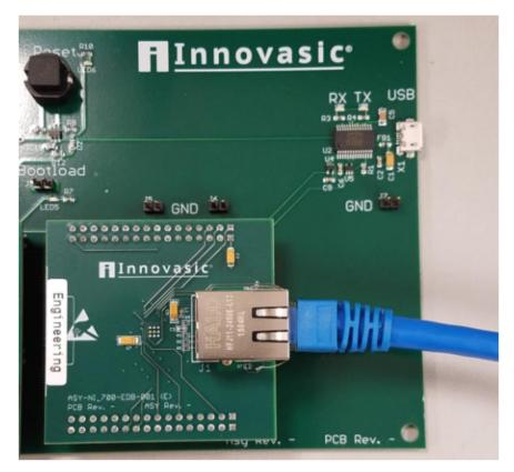
Figure 6 – Ethernet Personality Module Connection
