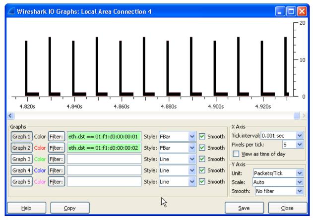
*Figure 38 – Wireshark Graph of the example schedule*
