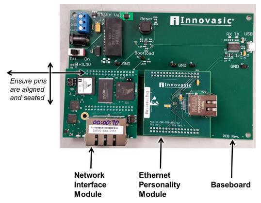
**Step 1:** Connect the Network Interface Module and the Ethernet Personality Module to the Network Interface Baseboard as shown in Figure 3.
