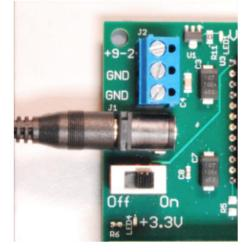
Figure 8 – Power ON Switch location
