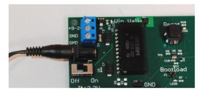
Figure 5 – Power Cable Connection
