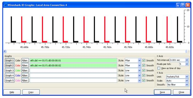
Figure 40 – Wireshark Graph of the modified schedule
