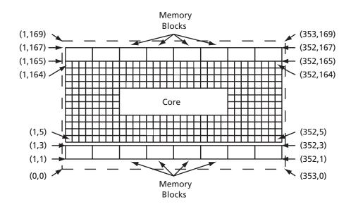
Figure 1-8 • Core Cell Coordinates for the APA1000
