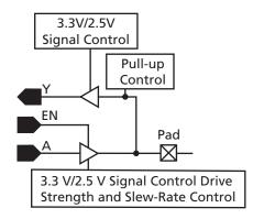
Figure 1-9 • I/O Block Schematic Representation
