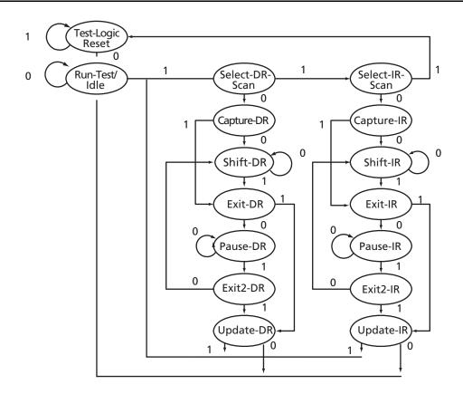
Figure 1-13 • TAP Controller State Diagram
