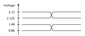
Figure 1-11 • LVPECL High and Low Threshold Values
