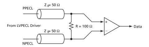
Figure 1-10 • Recommended Termination for LVPECL Inputs
