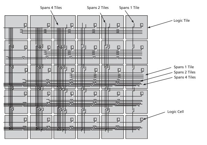
Figure 1-5 • Efficient Long-Line Resources
