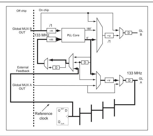
Figure 1-20 • Using the PLL for Clock Deskewing
