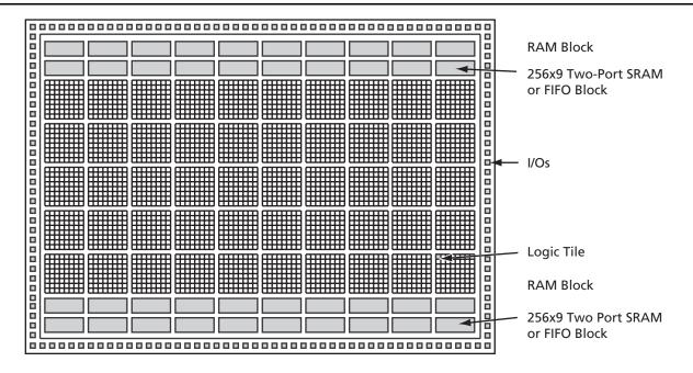
Figure 1-1 • The ProASICPLUS Device Architecture
