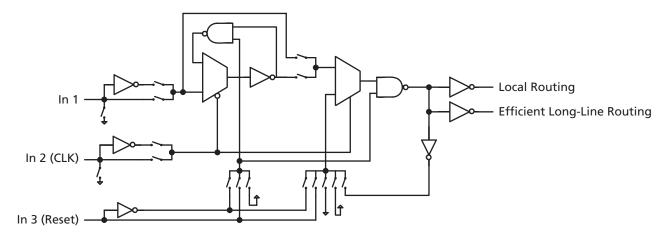
Figure 1-3 • Core Logic Tile
