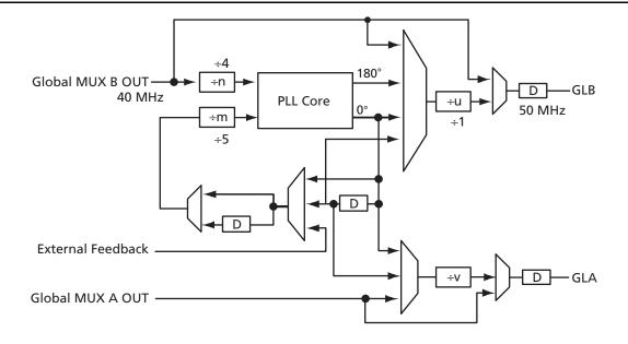
Figure 1-17 • Using the PLL 40 MHz In, 50 MHz Out
