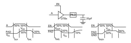
Figure 1-26 • Tristate Buffer Delays
