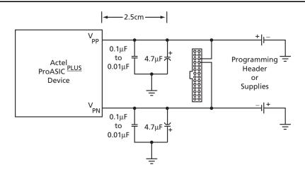
Figure 1-49 • ProASICPLUS V<sub>PP</sub> and V<sub>PN</sub> Capacitor Requirements
