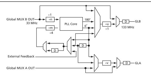
Figure 1-16 • Using the PLL 33 MHz In, 133 MHz Out
