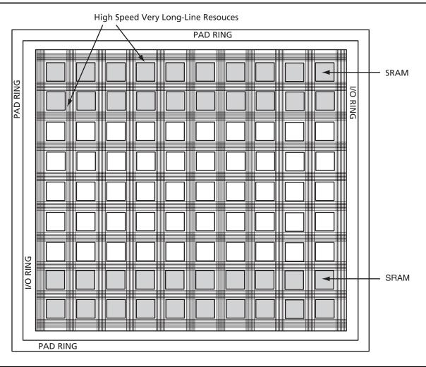
Figure 1-6 • High-Speed, Very Long-Line Resources
