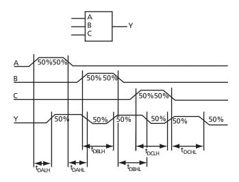
Figure 1-29 • Module Delays
