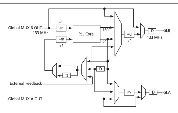
Figure 1-18 • Using the PLL to Delay the Input Clock
