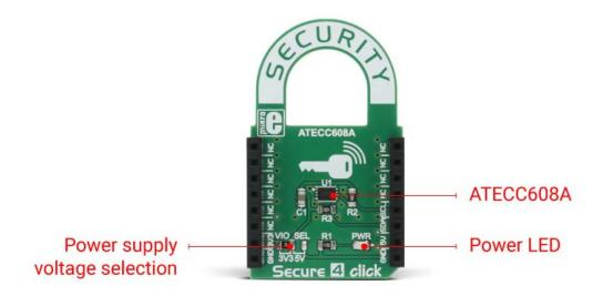
The device is consuming very low current, especially while it is in the sleep mode. The chip itself uses less than 150nA, in that case. The voltage range which can be used to power up the Security 4 click, allows for it to work with both 3.3V and 5V capable MCUs.
