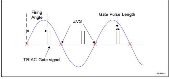
The MCU operation is synchronized with the voltage mains thanks to the zero-voltage switching (ZVS) signal. This signal is sent directly to an MCU input pin, which is set as external interrupt.
