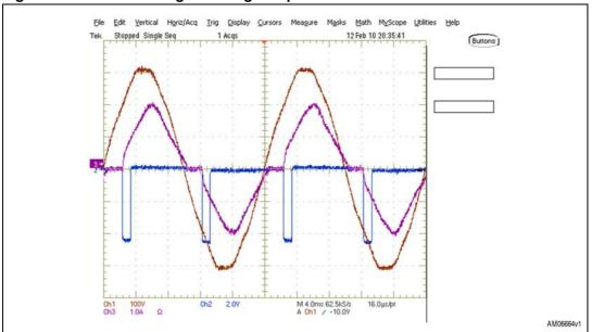
Figure 6. Motor working at the highest power level
