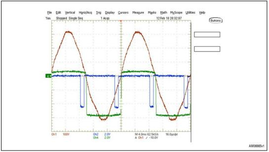
Figure 7. Zero-voltage switching (ZVS)
