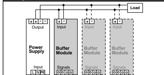
Buffer modules can be connected in parallel to increase the output ampacity or the hold-up time.
