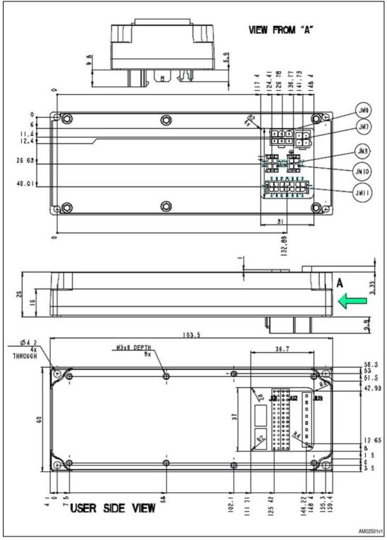
Figure 6. Mechanical data (dimensions in mm) continued
