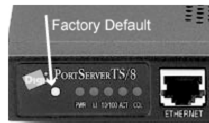
PortServer TS 8 Reset Button (Hold button down until LEDs flash 5-1-1 pattern)
