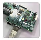
d. Connect Ethernet Cable to TX port of TX board
