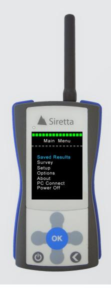
The menus and operation of the SNYPER-3G Spectrum have been designed to be completely intuitive, making the unit user friendly and with little referral to the User Guide necessary . A large high contrast LCD display ensures that all information is clear and visible, giving considerable data presentation simultaneously.
