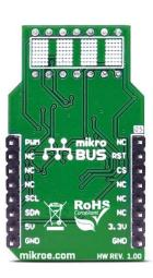
**4Dot-Matrix R click** allows you to display 4 characters of 5x7 dot size. The click is designed to run on either 3.3V or 5V power supply. It communicates with the target microcontroller over I2C interface, with additional functionality provided by the following pins on the mikroBUS™ line: RST, CS, PWM.
