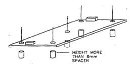
Please left 4mm space from the surfaces and the sides of PCB, especially from the solder surface, 8mm space is neccessary. If the space is not enough, the specification of insulation and withstand will not be satisfied.
