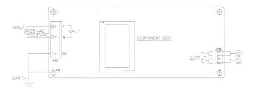
● Please use the following housings & pins to connect the input termina Connectors in use (Molex made)
