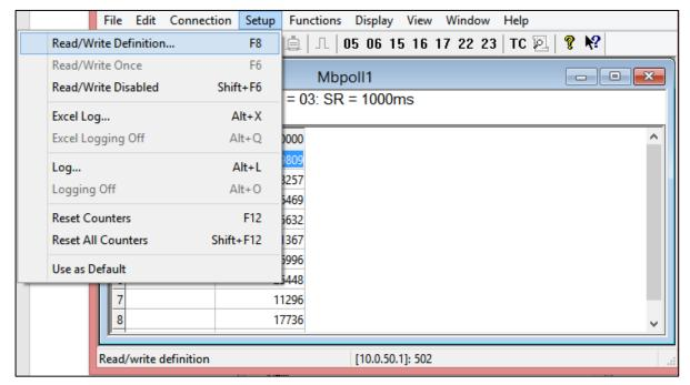
Figure 2.32 Modbus Poll Setup Read/Write Definition
