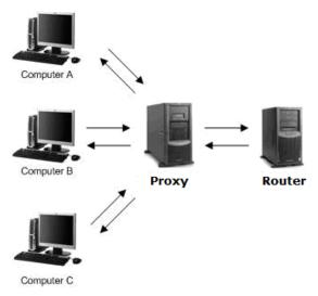
Figure 2.96 Example of IGMP Proxy
