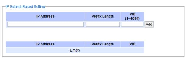
Figure 2.126 IP Subnet-Based VLAN Setting Webpage
