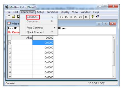
Figure 2.28 Entering Connection Setup Menu of the Modbus Poll
