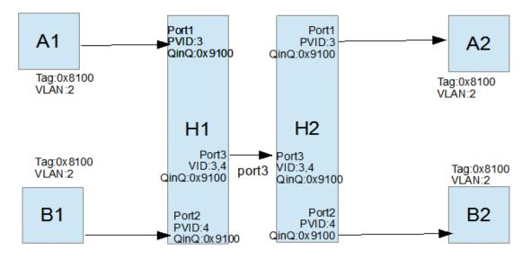
Figure 2.129 Example of QinQ Deployment
