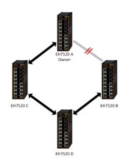
Figure 2.146 Example of Ring Topology for ERPS Setup (Example made on EH7520)
