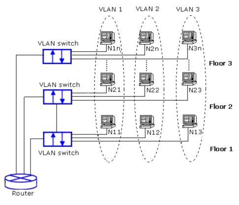
Figure 2.116 Example of VLAN Configuration
