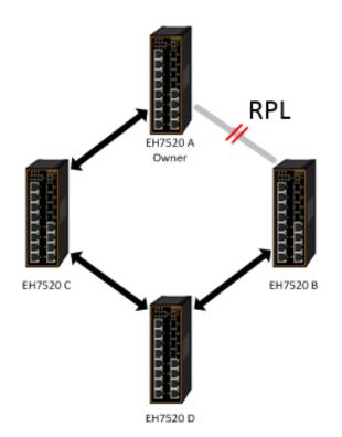
Figure 2.142 An Example of Ring Topology (Example made on EH7520)
