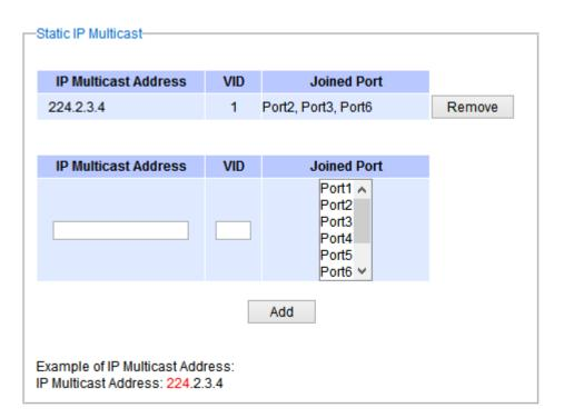
Figure 2.102 Example of Static IP Multicast Setting
