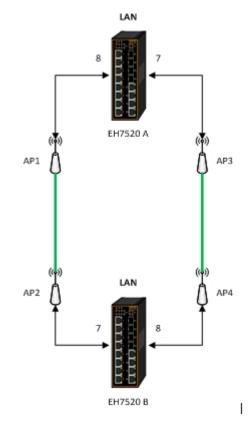
Figure 2.155 Example 2 of Two Wired Bridge U-ring (Example on EH7520)
