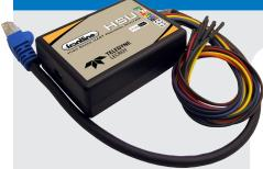
The Frontline HSU Protocol Analyzer includes powerful Frontline software and the High Speed UART hardware interface.
