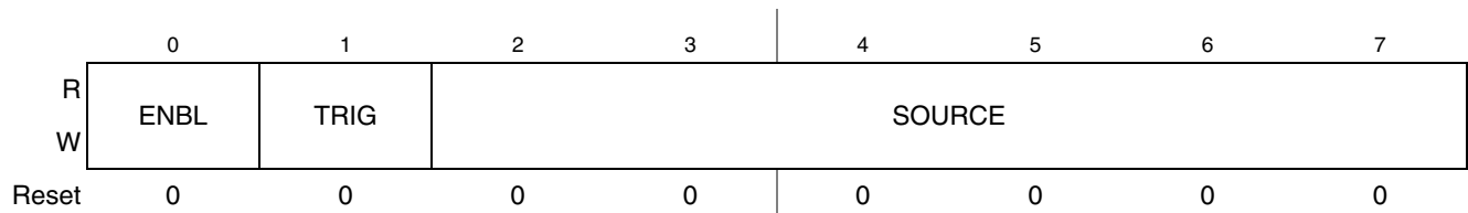
Figure 13-2. Channel Configuration Registers (CHCONFIG n )
