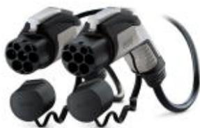
Mobile AC charging cable with Vehicle Connector and Infrastructure Plug, with locking option for U-lock, with protective caps, GB/T, GB/T 20234.2-2015, GB/T 18487.1-2015, 16 A / 440 V (AC), design line C-Line, cable: 5 m, black, straight, mating face: black, handle area: gray
