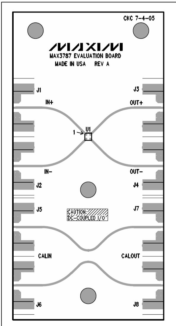
Figure 2. MAX3787 EV Kit Component Placement Guide—Component Side
