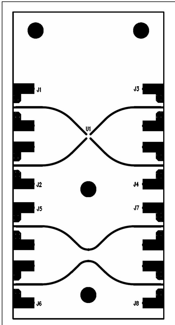
Figure 3. MAX3787 EV Kit PC Board Layout—Component Side
