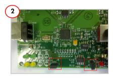
Place jumper on J5 (power status) and J6 (port status) to enable LEDs D1 and D3-D6. Power LED D1 glows only in self-powered mode. The green LEDs (D3 and D5) indicate that the downlink port is enabled. The amber LEDs (D4 and D6) indicate the port has an exception condition.
