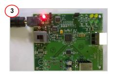
Plug the wall mounted power supply into an AC power receptacle providing power in the range 100 V to 240 V, 50 Hz or 60 Hz. Connect the power supply plug to the hub's 'DC Supply' jack J12.
