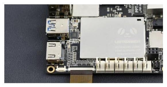
Note: The FPC must be fully inserted in the connector. If not fully inserted, the actuator will not close properly. Should this be the case, lift up the actuator and repeat the process (starting with Step 1 above)
