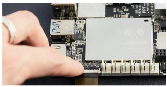
Insert the FPC of display part. Same as the main board part. Place the Golden Finger side down too.
