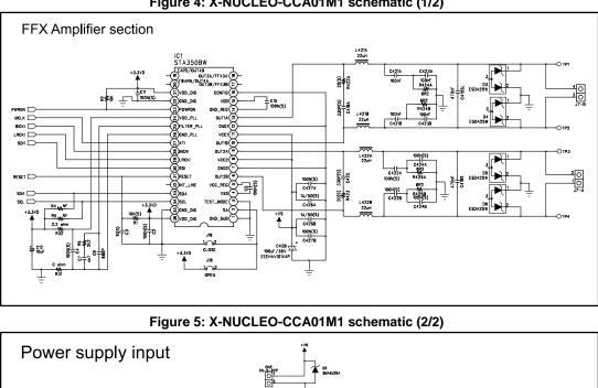
T The range of +Vs is from +5V to +26V
