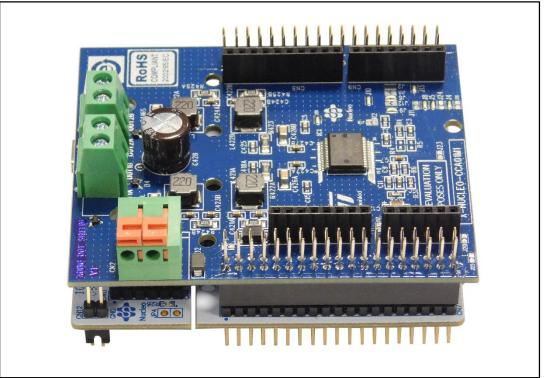
Figure 2: X-NUCLEO-CCA01M1 plugged on STM32 Nucleo board
